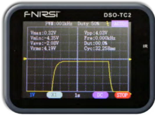
Figure 2 – Voltage change for fade on and off
