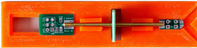
Figure 4 – Jig with components ready for soldering mast
