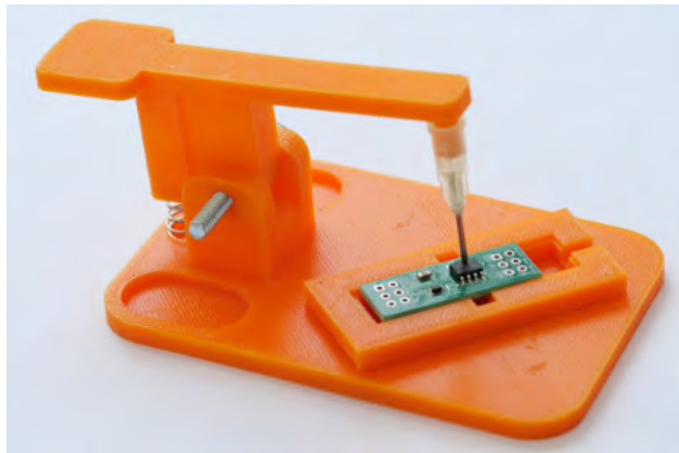
Figure 6 – Main board in its jig with third-hand soldering aid
