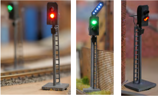
Figures 12,13,14 – Completed two-aspect signal, Completed signal with optional feather and another two-aspect in situ
