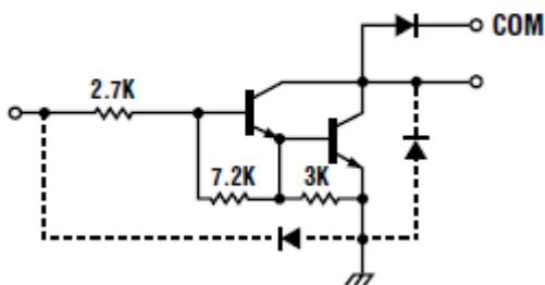
In electronics, the Darlington transistor is a semiconductor device which combines two bipolar transistors in tandem (often called a "Darlington pair") in a single device so that the current amplified by the first is amplified further by the
