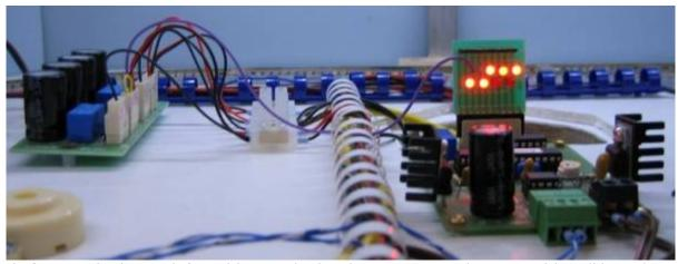
Instead of an LED in the top left position, a wire is taken to a PD3 point motor driver (kit 37a) and this controls both Kato points on the demonstration layout.
